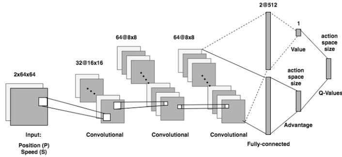
Fig. 2: The architecture of the Deep Neural Network.
